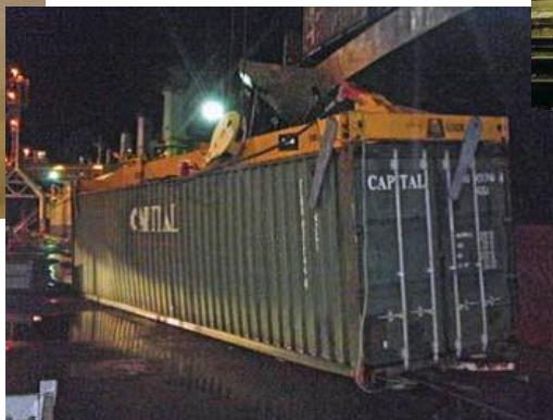
Darwin – Misdeclared container falls (narrowly missing 2 people) after it exceeded the crane limit
