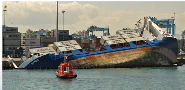
MV Deneb in 2011, rolled over after loading containers where [only] 1 in 10 varied between 1.9 to 6.7 times the declared weight
